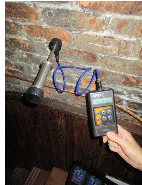
Photo 82 Brick moisture testing using a Tramex MRH III with 1 1/2-inch masonry pin probes.
