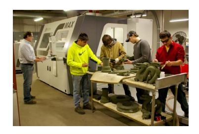
Largest printable area available in any 3D printer in North America and can produce molds for virtually any metal alloy
