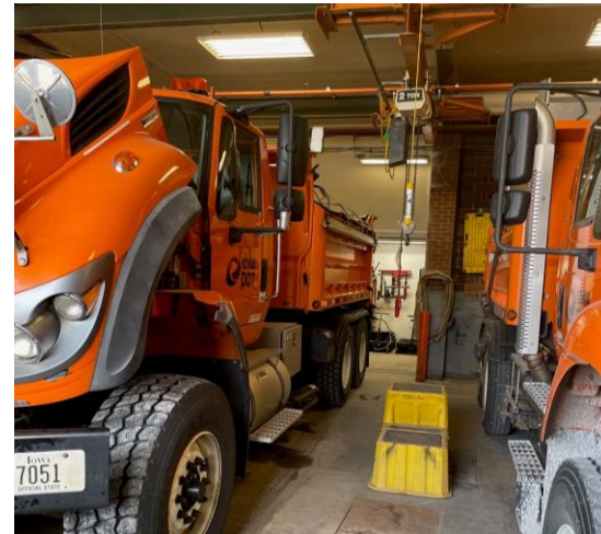
Insufficient safe space to maintain and operate attachments such as wing plows between trucks.
