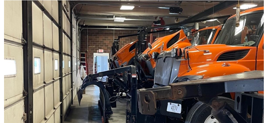
Limited clearance with plow attachment.
