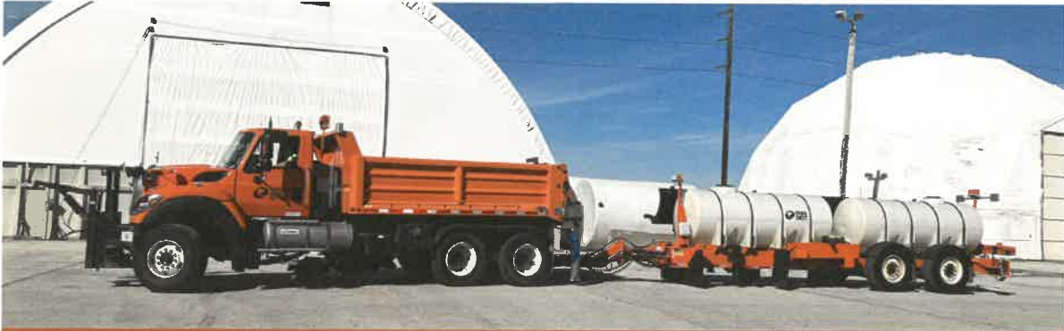
Tow plow truck fully deployed on a heavy duty truck.
