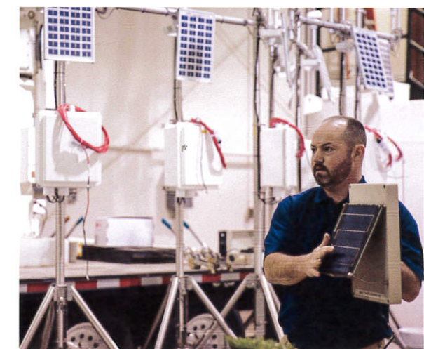
IFC Research Engineer Tony Loeser shows off one of the IFC's network of 250+ stream sensors.
