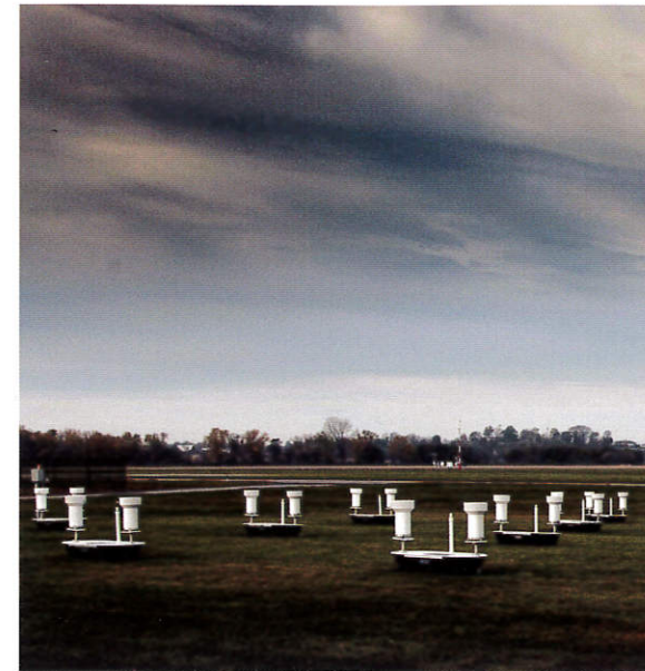
IFC rain gauges prepared for deployment during the NASA field campaign in the Turkey River Watershed.
