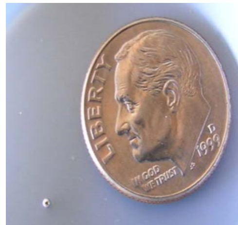
Figure 3. Amount of mercury (lower left) in an average CFL relative to a dime.
