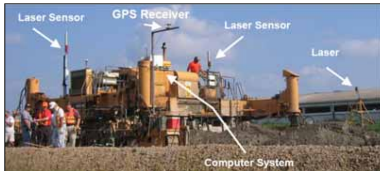
Slipform Paving Machine with GPS Guidance Equipment Attached
