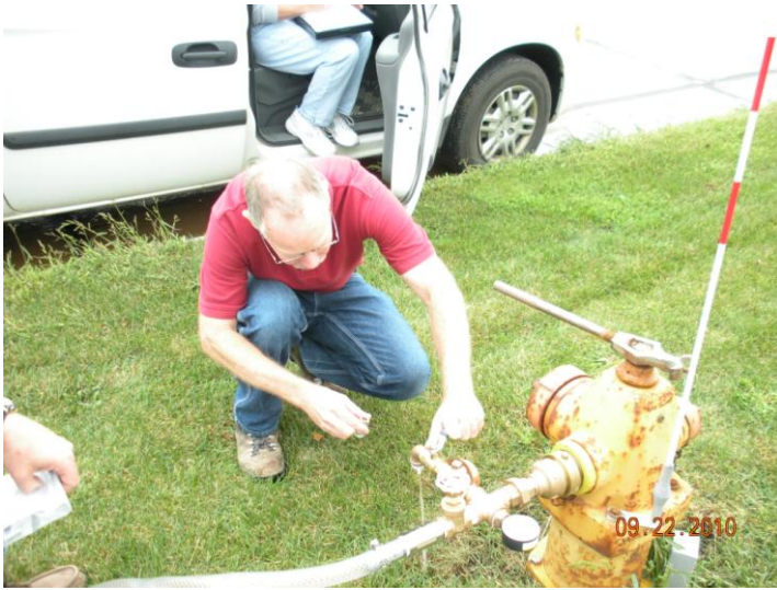
Multi-state AWOP Training Event: Using a hydrant sampler for mapping the chlorine levels in the distribution system
