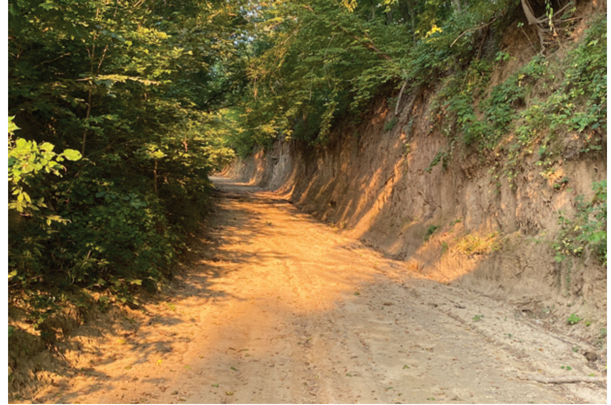
FIGURE 1 (LEFT). Loess (wind-blown silt) has the unique property of maintaining its continuity when exposed in near vertical faces.
