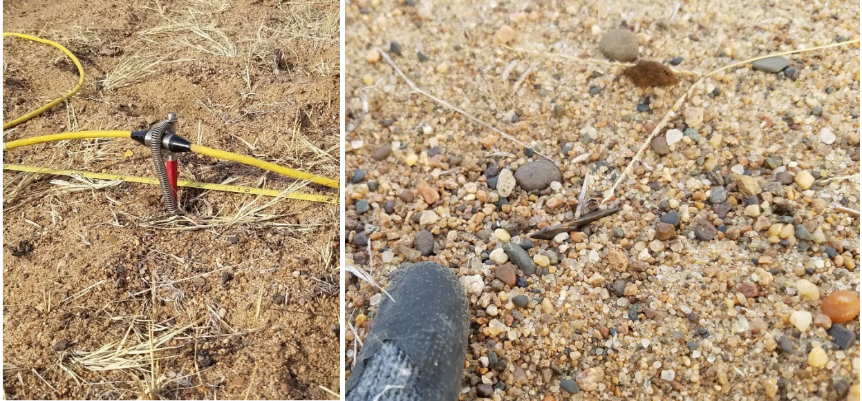
Figure 18. Left: An electrode stake installed in the coarse sand found along Site B Top. Right: A close-up photo with a finger for scale showing the coarse sand and gravel along Site B Top.
