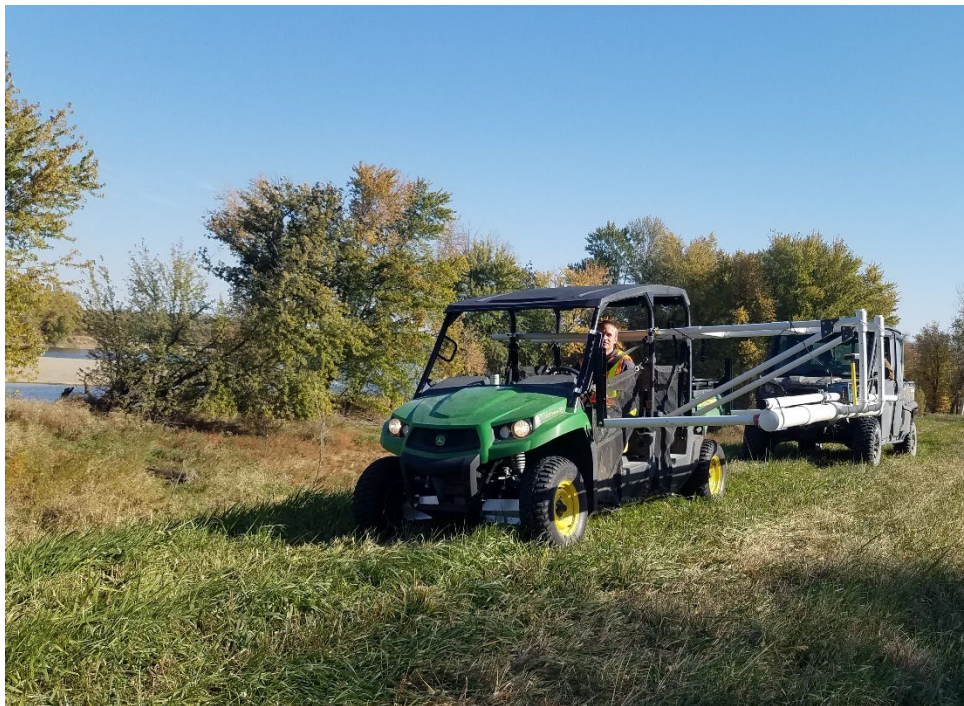
Figure 1. EM data collection at one of the levee sites.
