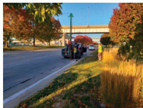
FIGURES 2 AND 3. Soil cores are collected beneath a major street in Des Moines to identify native settlement locations prior to European settlement.
