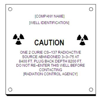
The size of the plaque should be convenient for use on active or inactive wells, e.g., a 7-inch square. Letter size of the word "CAUTION" should be approximately twice the letter size of the rest of the information, e.g., ½-inch and ¼-inch letter size, respectively.
