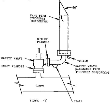
**92.7(5)** The safety valve capacity of each boiler shall be such that the safety valve or valves will discharge all the steam that can be generated by the boiler without allowing the pressure to rise more than 5 percent above the highest pressure to which any valve is set and in no case to more than 6 percent above maximum allowable working pressure.
