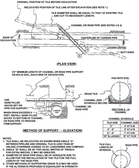
IF THE ALTERNATE PROPOSED IS EQUIVALENT IN STRENGT TO THE CHANNEL SECTIONS SHOWN AND IF APPROVED BY THE LANDOWNER.
