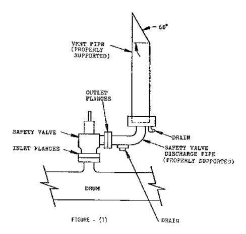
**92.7(5)** The safety valve capacity of each boiler shall be such that the safety valve or valves will discharge all the steam that can be generated by the boiler without allowing the pressure to rise more
