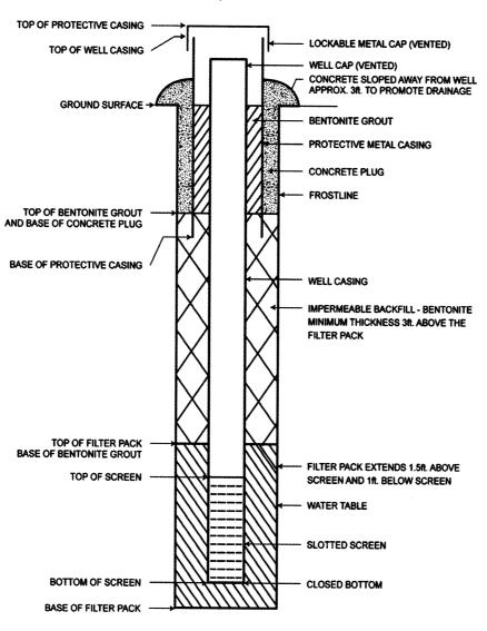
Figure 1 Typical Monitoring Well Cross Section
