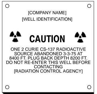
The size of the plaque should be convenient for use on active or inactive wells, e.g., a 7-inch square. Letter size of the word "CAUTION" should be approximately twice the letter size of the rest of the information, e.g., ½-inch and ¼-inch letter size, respectively.
