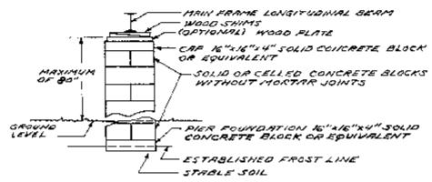
FIGURE 2 - PIERS OVER 40" IN HEIGHT AND NOT <u>EXCEPDING 80" IN HEIGHT</u> (POUBLE BLOCK CONSTRUCTION)
