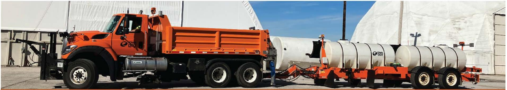
Tow plow truck fully deployed on a heavy duty truck.
