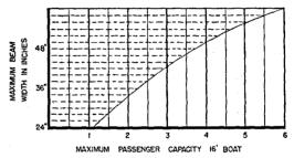
BASE WEIGHT 325 LBS INCLUDES MOTOR & MISC GEAR Passenger capacities of canoes for hire shall
